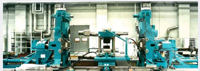
Universal mill stand in roll changing device, vertical and horizontal rolls disassembled
