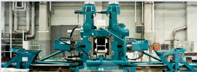
Universal mill stand in roll changing device
